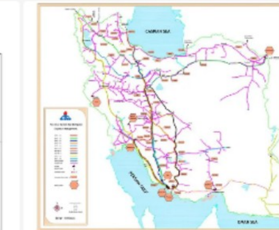
Fig. 1 Iran's gas supply system, showing the location of main cities, pipelines, compressor stations, and high-pressure gas pipelines
